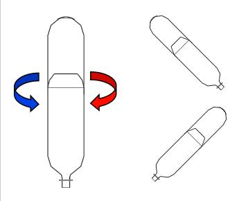
**Step 3:** Rotate and observe your water rocket from several angles to ensure good alignment.
