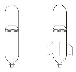
**Step 4:** Tape/secure the joint between the nose cone stage and the pressure vessel.
