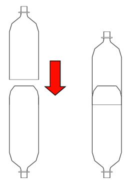
**Step 2:** Carefully align top portion of bottle on the 2L bottle to be used for the pressure vessel.
