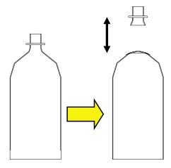
Option 1: A) The neck can be cut off of the top of the nose cone as shown in Step 4. This will slightly improve the aerodynamics of the rocket. B) The resulting hole can simply be covered with tape. (Use a hack saw blade for cutting through the thicker material at the neck of bottle. Utility and other knives are NOT recommended for this process.)
