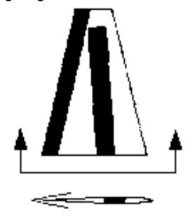
**Note**: Adding clear packing tape keeps the leading edge from curling up and mounting tape adds strength and stiffness to the fin.
