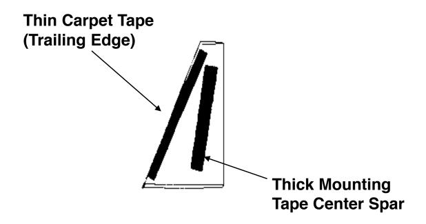
5. Trim to desired sweep, add clear packing tape over trailing edge.
